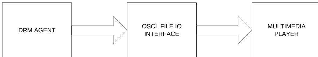
Figure 3: Data Interactions for Wrapped DRM.
