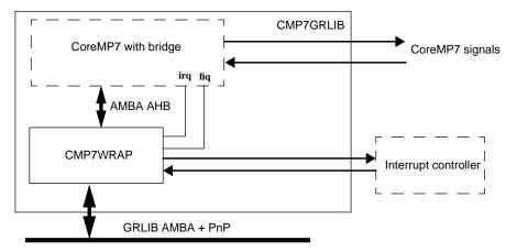
Figure 75. Block diagram
