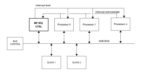
Figure 165. LEON3 multiprocessor system with Multiprocessor Interrupt controller
