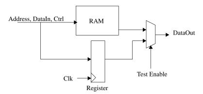
Figure 258. Scan test support
