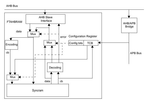
Figure 90. Block diagram
