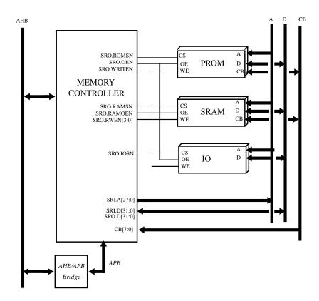
Figure 111. 32-bit FT PROM/SRAM/IO controller
