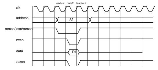
Figure 214. Write cycle with BEXCN. Chip-select (iosn) is not asserted in lead-in cycle for io-accesses.
