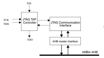
Figure 8. JTAG Debug link block diagram
