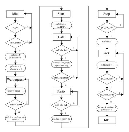
Figure 25. Flow chart for the transmitter state machine
