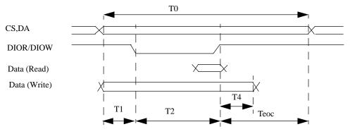
Figure 37. PIO timing diagram.
