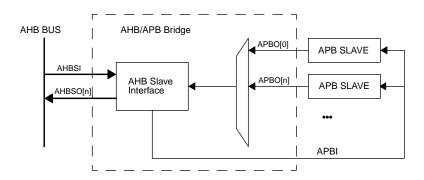
Figure 20. AHB/APB bridge block diagram
