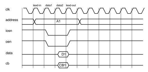
Figure 205. I/O read cycle (0-waitstates)
