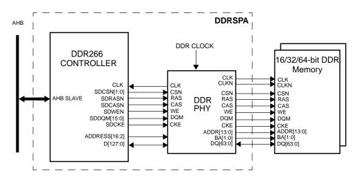
Figure 77. DDRSPA Memory controller conected to AMBA bus and DDR SDRAM
