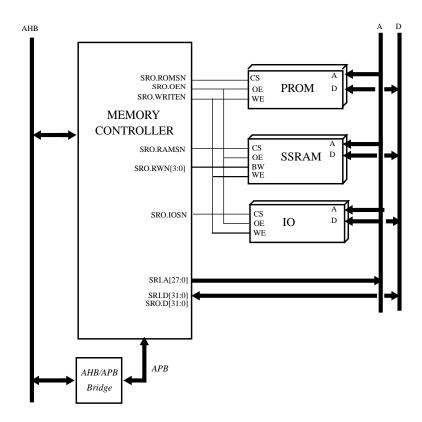
Figure 249. 32-bit SSRAM/PROM/IO controller
