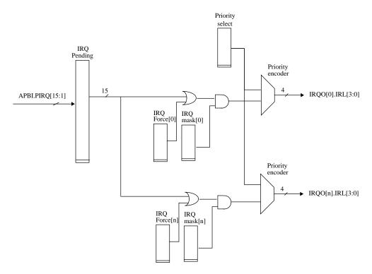
Figure 166. Interrupt controller block diagram
