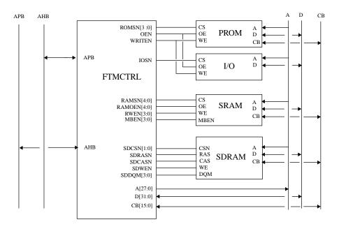
Figure 91. FTMCTRL connected to different types of memory devices
