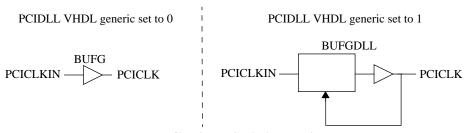
Figure 63. Virtex PCI clock generation
