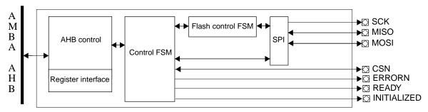
Figure 245. Block diagram
