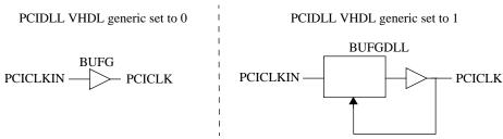
Figure 74. Virtex 5 PCI clock generation
