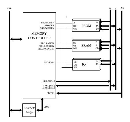
Figure 246. 8/32-bit PROM/SRAM/IO controller
