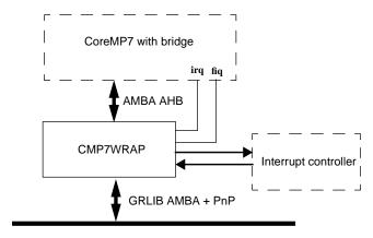
Figure 76. Block diagram
