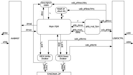
Figure 261. Block diagram of the internal structure of the GRUSBDCL. Blocks with rounded corners are implemented as VHDL procdures while squares represent VHDL entities.
