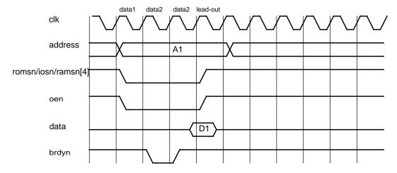
Figure 103. READ cycle with one extra data2 cycle added with BRDYN (synchronous sampling). Lead-out cycle is only applicable for I/O accesses.
