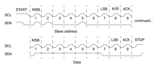
Figure 162. Complete I<sup>2</sup>C data transfer
