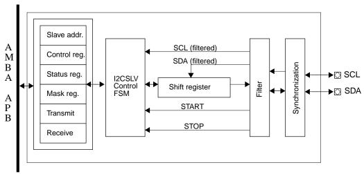
Figure 163. Block diagram
