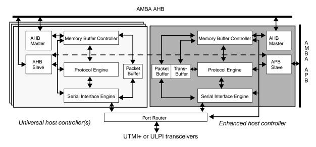
Figure 160. Block diagram of both host controller types
