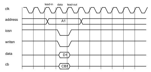
Figure 98. I/O write cycle (0-waitstates)
