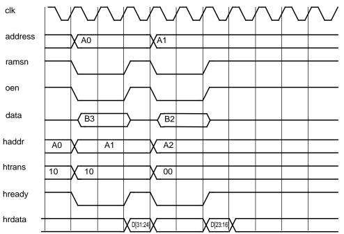
Figure 129. 8-bit SRAM non-sequential read access with 0 wait-states and EDAC enabled.
