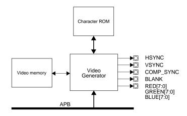
Figure 32. APBVGA block diagram
