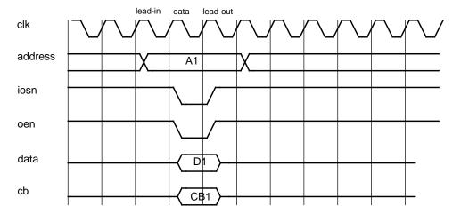
Figure 206. I/O write cycle (0-waitstates)
