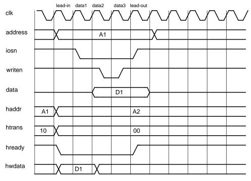
Figure 122. I/O write access with 0 wait-states.
