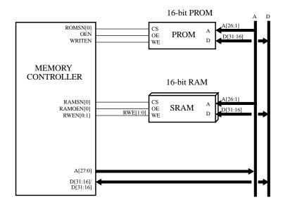
Figure 102. 16-bit memory interface example
