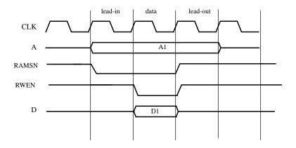
Figure 248. 32-bit PROM/SRAM/IO write cycle
