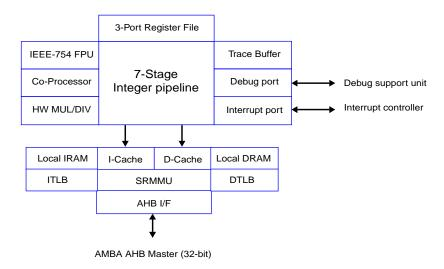
Figure 176. LEON3 processor core block diagram
