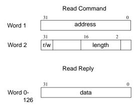
Figure 264. Layout of USBDCL read commands and replies.
