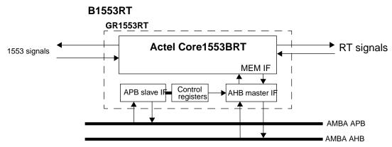
Figure 43. B1553RT block diagram
