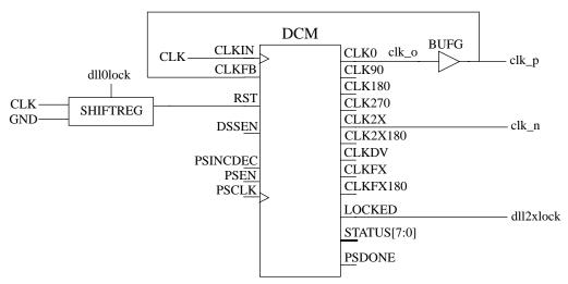
Figure 65. Virtex 2/4 generation of CLK2X clock when VHDL generic clk2xen is non-zero
