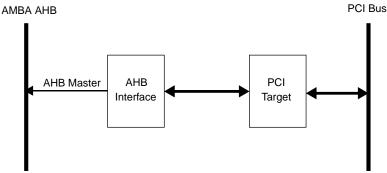
Figure 236. Target-only PCI interface
