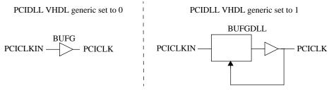
Figure 69. Virtex 2/4 PCI clock generation
