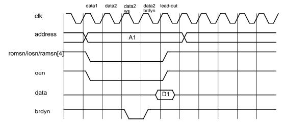
Figure 105. Read cycle with one waitstate (configured) and one BRDYN generated waitstate (synchronous sampling).
