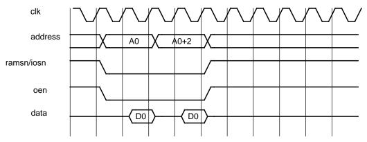
Figure 254. 32-bit PROM/IO read cycle in 16-bit mode
