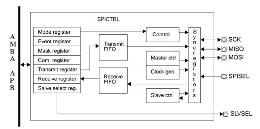
Figure 243. Block diagram
