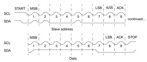
Figure 164. Complete I<sup>2</sup>C data transfer
