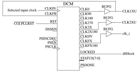
Figure 54. Spartan 3/e generation of main clock
