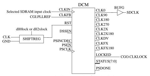
Figure 73. Virtex 5 generation of SDRAM clock
