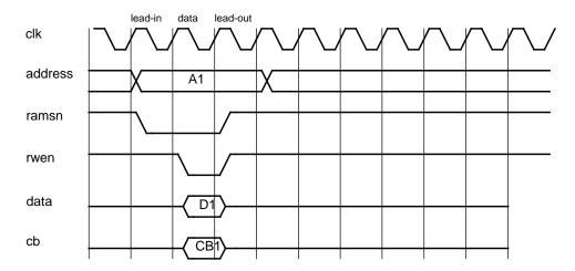
Figure 208. Sram write cycle (0-waitstates)
