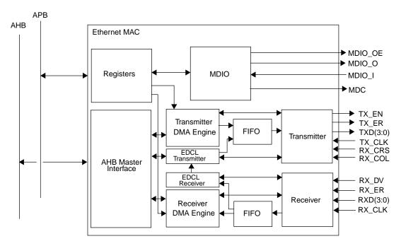
Figure 137. Block diagram of the internal structure of the GRETH.
