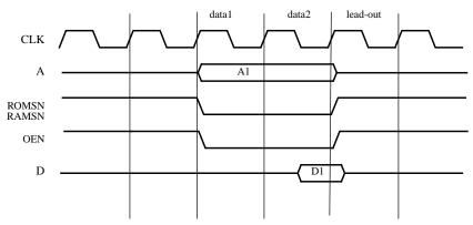
Figure 247. 32-bit PROM/SRAM/IO read cycle
