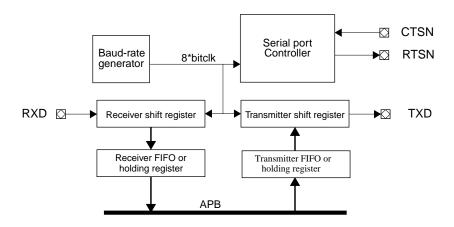
Figure 30. Block diagram
