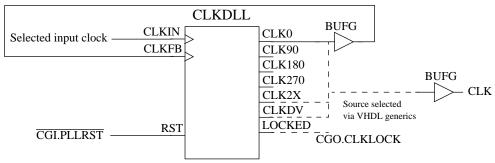
Figure 61. Virtex generation of main clock
