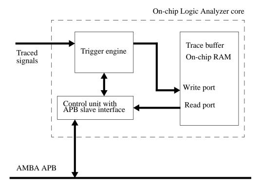
Figure 191. On-chip Logic Analyzer block diagram
