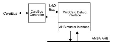
Figure 265. WildCard Debug Interface block diagram
