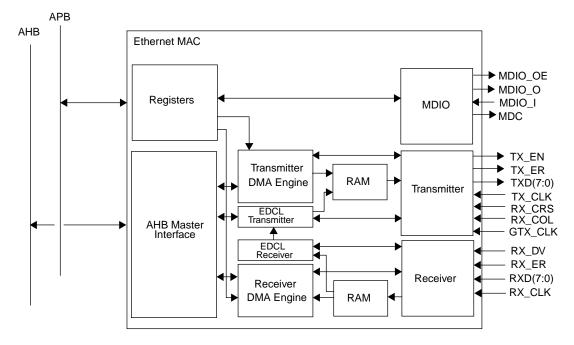
Figure 138. Block diagram of the internal structure of the GRETH\_GBIT.
