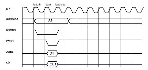
Figure 100. Sram write cycle (0-waitstates)
