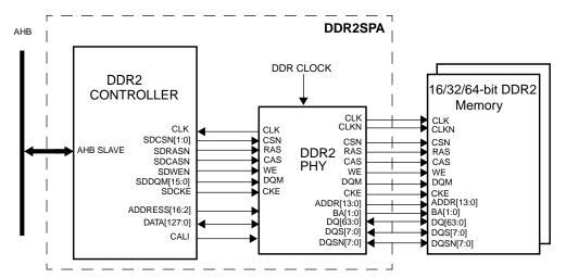
Figure 78. DDR2SPA Memory controller connected to AMBA bus and DDR2 SDRAM
