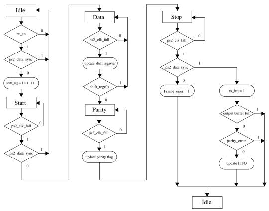
Figure 24. Flow chart for the receiver state machine
