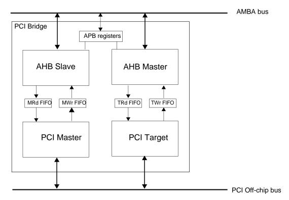
Figure 215. GRPCI master/target
