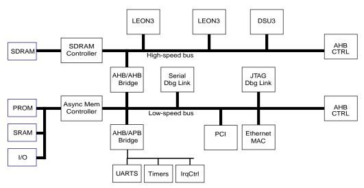
Figure 2. LEON3 system with a bi-directional AHB/AHB bridge
