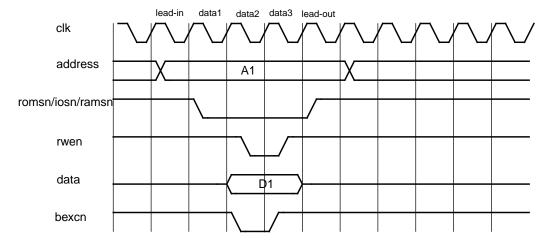
Figure 113. Write cycle with BEXCN.
