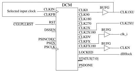
Figure 70. Virtex 5 generation of main clock
