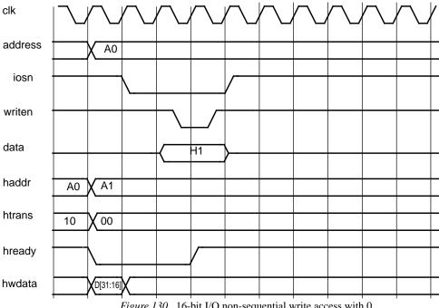
Figure 130. 16-bit I/O non-sequential write access with 0 wait-states.
