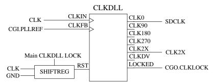
Figure 62. Virtex generation of SDRAM clock with feedback clock enabled
