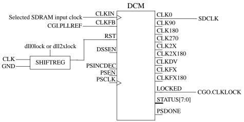
Figure 59. Spartan 3/e generation of SDRAM clock
