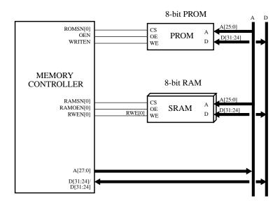
Figure 101. 8-bit memory interface example
