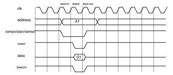
Figure 107. Write cycle with BEXCN. Chip-select (iosn) is not asserted in lead-in cycle for io-accesses.
