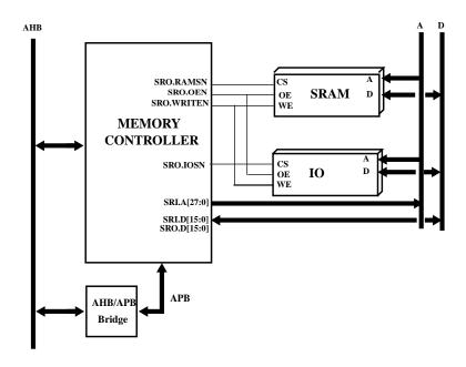
Figure 124. Block diagram
