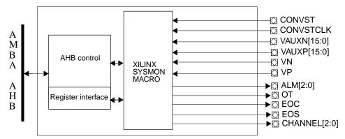
Figure 155. Block diagram
