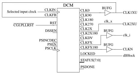
Figure 64. Virtex 2/4 generation of main clock
