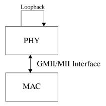
Figure 238. Block diagram of the PHY simulation model connected to a MAC.
