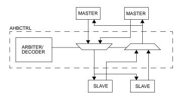
Figure 3. AHB controller block diagram
