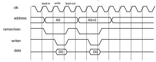
Figure 255. 32-bit PROM/IO write cycle in 16-bit mode
