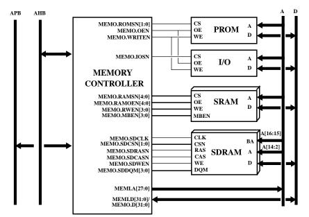
Figure 199. Memory controller conected to AMBA bus and different types of memory devices
