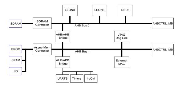
Figure 5. System with multiple AHB buses
