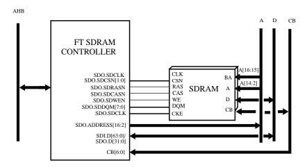
Figure 108. FT SDRAM memory controller connected to AMBA bus and SDRAM
