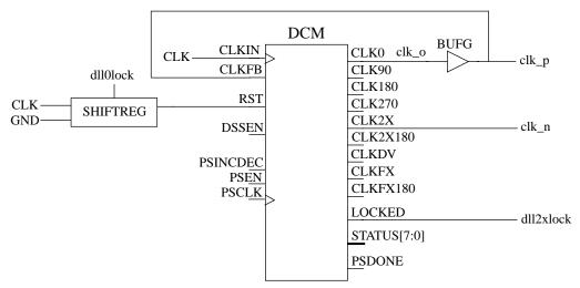
Figure 71. Virtex 5 generation of CLK2X clock when VHDL generic clk2xen is non-zero
