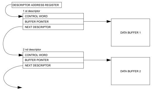
Figure 158. Example of the structure of a DMA descriptor linked list in memory.
