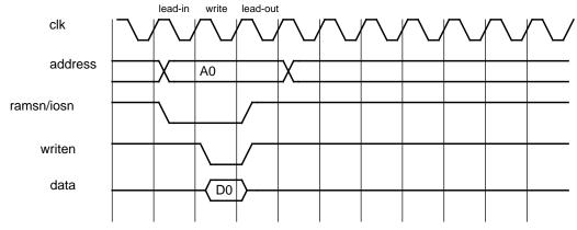
Figure 253. 32-bit PROM/IO write cycle
