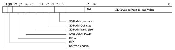
Figure 109. SDRAM configuration register
