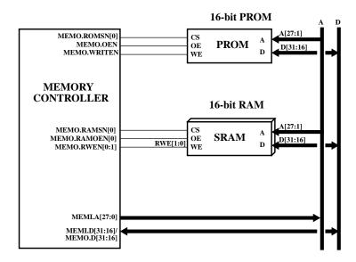
Figure 210. 16-bit memory interface example
