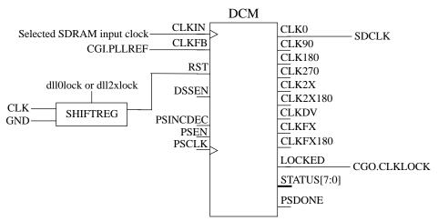
Figure 68. Virtex 2/4 generation of SDRAM clock
