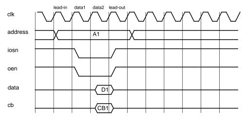
Figure 97. I/O read cycle (0-waitstates)
