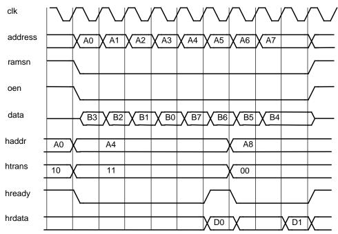
Figure 126. 32-bit SRAM sequential read accesses with 0 wait-states and EDAC enabled.
