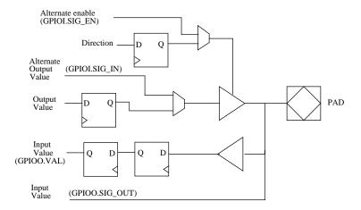
Figure 144. General Purpose I/O Port diagram
