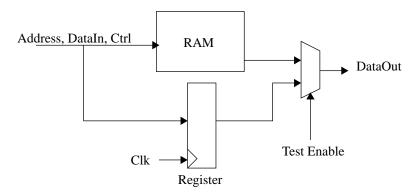
Figure 257. Scan test support
