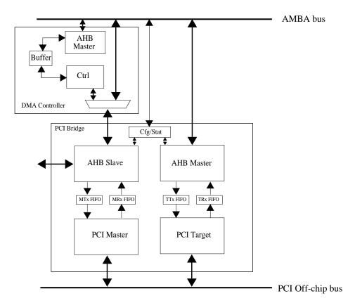
Figure 231. DMA Controller unit
