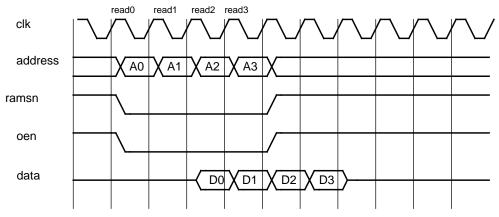
Figure 250. 32-bit SSRAM read cycle
