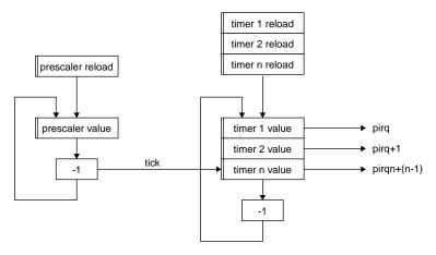
Figure 132. General Purpose Timer Unit block diagram
