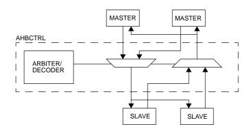
Figure 6. AHB controller block diagram
