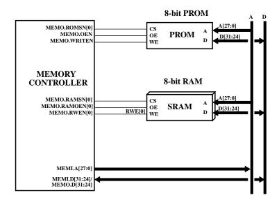
Figure 209. 8-bit memory interface example
