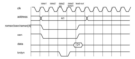
Figure 212. Read cycle with one waitstate (configured) and one BRDYN generated waitstate (synchronous sampling).
