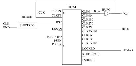
Figure 55. Spartan 3/e generation of CLK2X clock when VHDL generic clk2xen is non-zero
