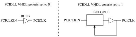
Figure 60. Spartan 3/e PCI clock generation
