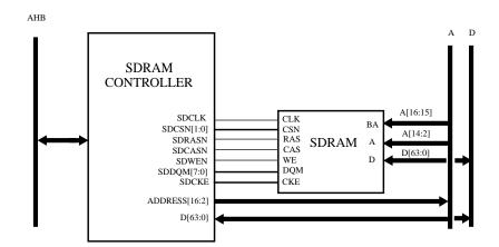
Figure 242. SDRAM Memory controller connected to AMBA bus and SDRAM
