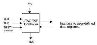
Figure 259. TAP controller block diagram
