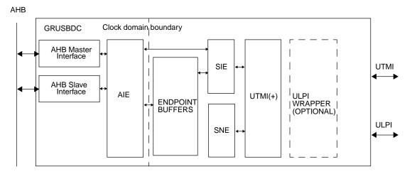
Figure 157. Block diagram of the internal structure of the core.
