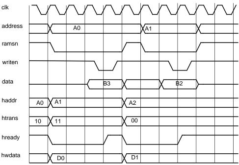
Figure 128. 8-bit SRAM non-sequential write access with 0 wait-states and EDAC enabled.
