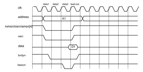
Figure 104. BRDYN (asynchronous) sampling and BEXCN timing. Lead-out cycle is only applicable for I/O-accesses.
