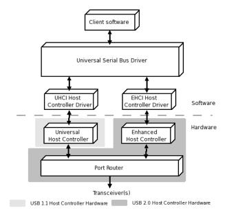
Figure 159. Block diagram of USB 2.0 host system
