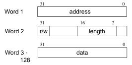
Figure 263. Layout of USBDCL write commands.
