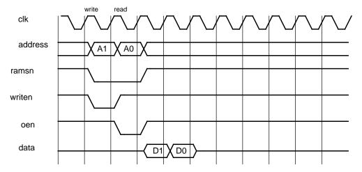
Figure 251. 32-bit SSRAM write cycle
