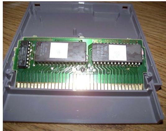
Figure 4-4. Inside a NES cartridge [38].
